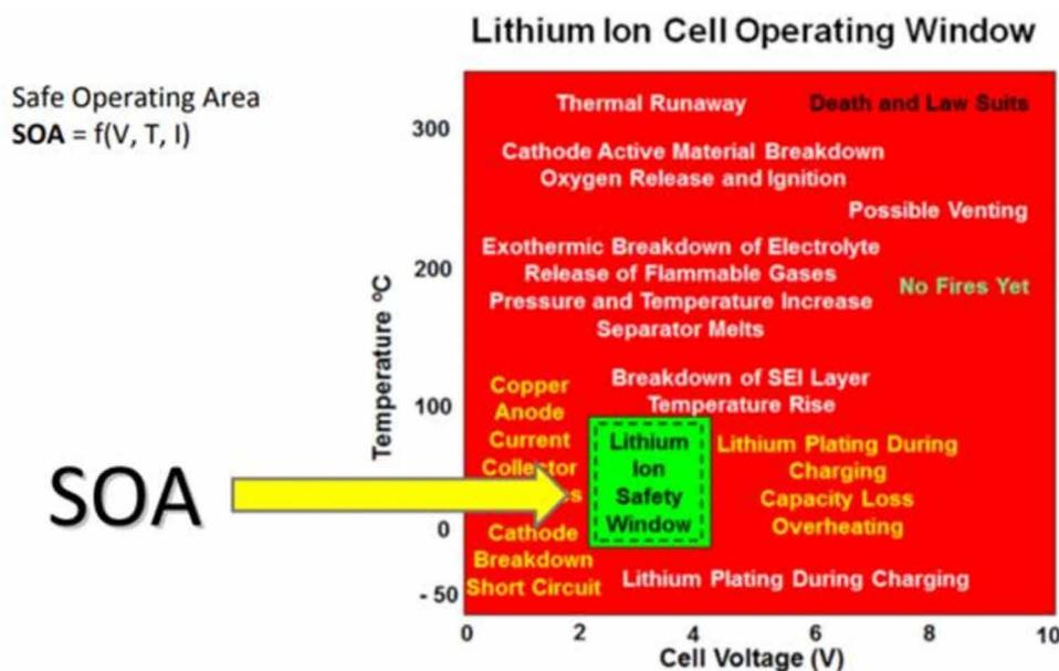
Performance of battery is an important parameter in a battery management system (BMS). The battery protection management involves two specific protection parameters i.e. electrical and thermal protection. The electrical protection helps the battery from getting damage i.e. its use outside the surface operating area, while the thermal protection helps to control the passive/active temperature and maintain its surface of operating area.
