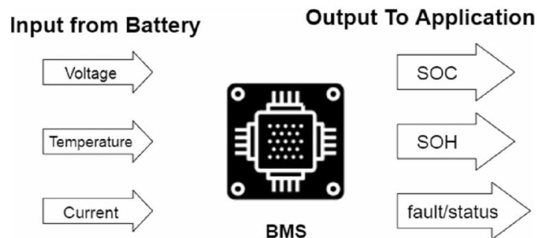
Monitoring and control are applied to all individual cells known as modules. Lithium-ion batteries are rechargeable having maximum energy density. These batteries are considered as standard choice for many appliances such as laptop, mobiles, electric vehicles etc. Their operations are in safe mode but it is critical during charging and discharging mode. If the voltage and current of any battery goes beyond
