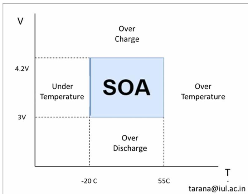
Figure 15. Temperature range for charging/discharging of battery.
